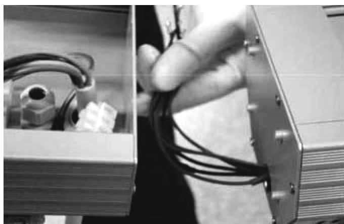
9 Remove interior end plate from heater: 6 Phillips screws fasten the heater body end plate in place:
