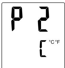
The current unit will be shown and the secondary display value will be flashing to indicate that the value can be changed. Rotate the control knob to change the value between Celsius and Fahrenheit.
