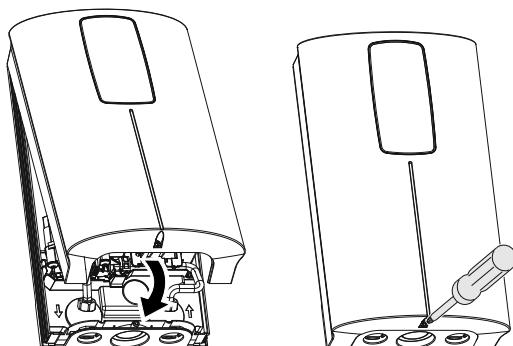
**9** Secure the cover with the screw.
