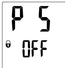
If the display-lock parameter is set to "On" and the user either holds the Information button for 5 seconds or lets the display time out for 15 seconds, the display-lock will become active.
