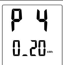
The secondary display will be flashing to indicate that the value can be changed by rotating the control knob. Consult your electricity bill to determine the cost of electricity per kWh.
