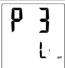
The current volume unit will be displayed and the value will be flashing to indicate that it can be changed. Rotate the control knob to change the value between liters and gallons.
