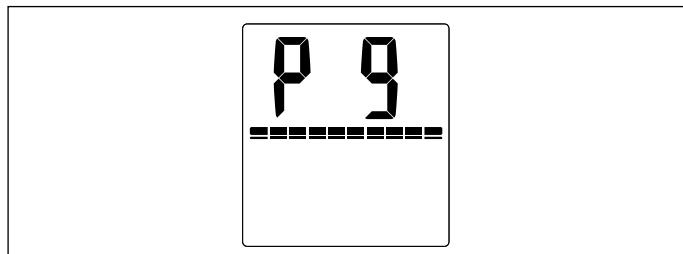
The power capacity status bar indicates the brightness setting. A full capacity bar indicates that the brightness is at the high setting. Two capacity bar segments indicates that the brightness is at the low setting.
