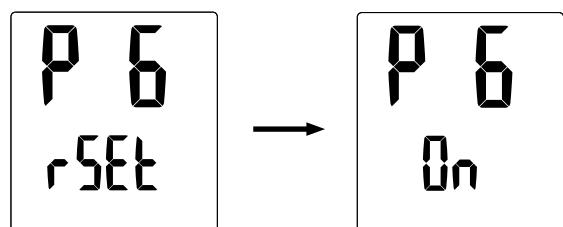
The display will be flashing to indicate that the value can be changed by rotating the control knob. When the value is set to "On", the reset must be confirmed by holding both Button 1 and Button 2 simultaneously for 5 seconds.
