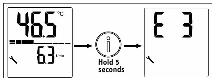
While the wrench is showing, press and hold the Information button for five seconds to advance the display to the error display page.
